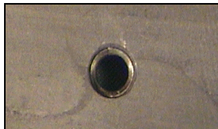
Figure 12: Proper HeliCoil Position
