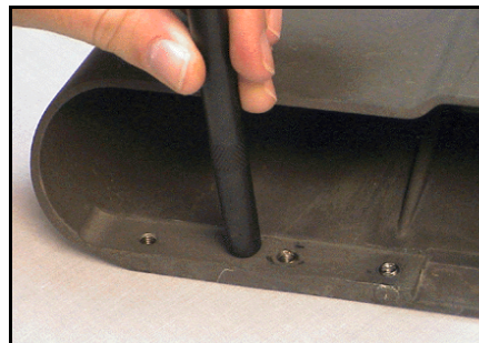
Figure 10: HeliCoil Tool in Place
