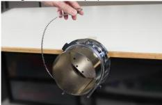
3. Place a piece of cap backing over the gauge and the teeth of the cap frame. Make sure that the backing is long enough to support the full embroidery area. For most wide angle cap frames a length of 16" will be enough.
