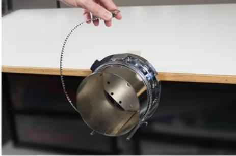
3. Place a piece of cap backing over the gauge and the teeth of the cap frame. Make sure that the backing is long enough to support the full embroidery area. For most wide angle cap frames a length of 16" will be enough.
