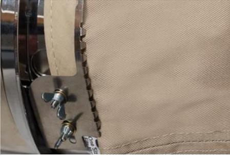
9. Continue bringing the strap around the front of the cap. On the front of the cap, the teeth of the strap must fall into the seam for the bill.
