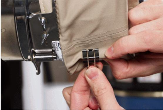
*These are only necessary when sewing the sides of the cap or if the cap is unstructured.*
