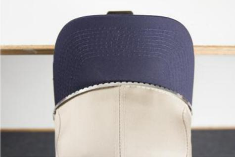
10. Bring the strap down the other side of the cap. Make sure the teeth of the strap fall just above the stitching attaching the sweat band. This will help ensure a level sewout.
