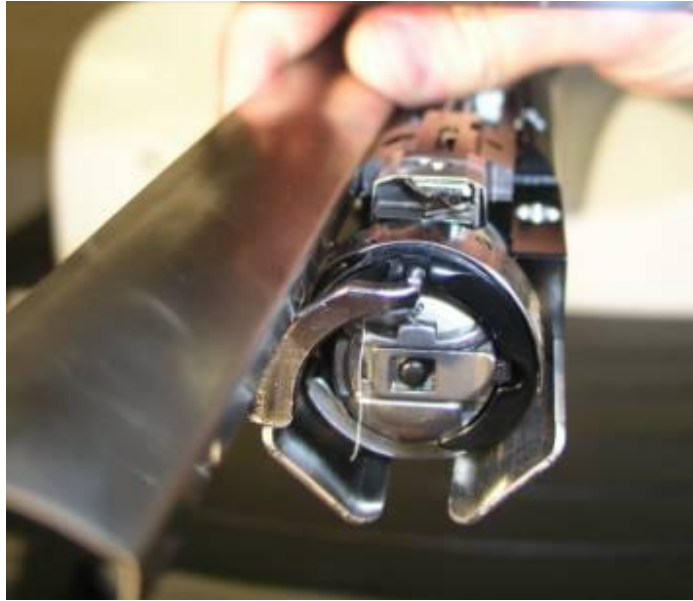
Figure 7: Trimmer Housing Alignment
