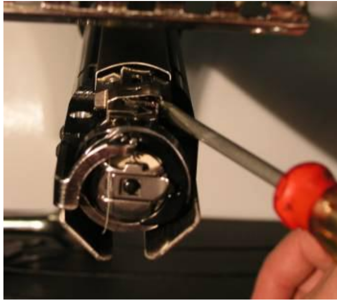
Figure 3: Removal of Knife Hold Down Clip
