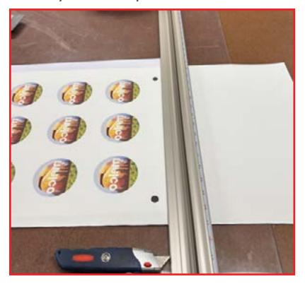
Cut the dye sublimated piece down to size and remove the cut registration dots from the twill.
