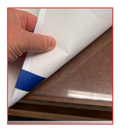
Put the combined piece with dye sublimated print on the top onto the heat press. Heat on the press should be set to 400 degrees Fahrenheit, time to 40 seconds, and pressure set to high. Close heat to sublimate.
