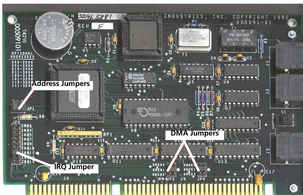
The I/O base jumpers (JP1 with numbers 2, 1, and 0 above each jumper) are located above the IRQ jumper.
