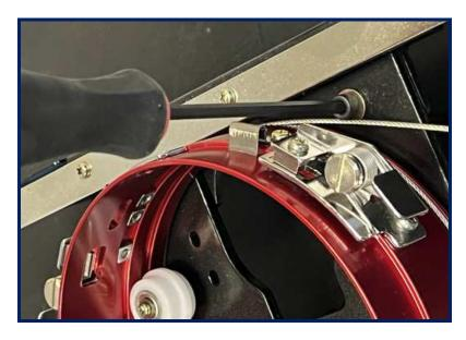
8. Route the Cable around the white Guides Wheels on the right and left side of the Bearing Plate. Install the Cable Studs into the black tabs on the Bearing Mounting Bracket as shown below and attach the Cable Tensioning Nuts.
