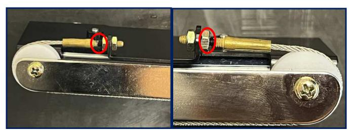
2. Place tape on the two opposite sides of the red Cylinder to prevent the Cable from unwinding.
