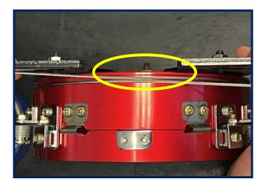
6. Position the new Bearing Mounting Bracket provided in the Upgrade Kit so that the cable crossing, Locator and center screw are all aligned as shown below. Make sure the Cable is in the groove on the red Cylinder.
